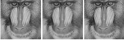
Fig. 2. Image deblurring with TV prior. (left) Original image, (middle) noisy and blurred image and (right) MMSE estimate computed with SGS.
