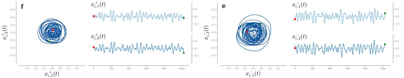
**Fig. 1.** (a) Partially elliptically polarized signal of Sec. 4.1 obtained by spectral synthesis, which is used in all subsequent simulations; (b) total PSD and polarization parameters used in (a); (c) and (d) uncorrelated orthogonally polarized components along  $\mu_x(\nu)$  and  $-\mu_x(\nu)$ ; (e) and (f) orthogonal circularly polarized components, also known as rotary components.
